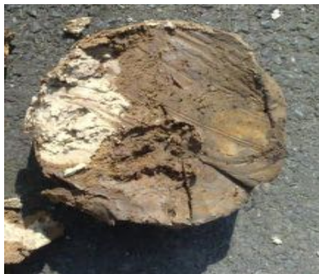
Figure 7 - Borehole Core. Showing Bentonite Plugging.
